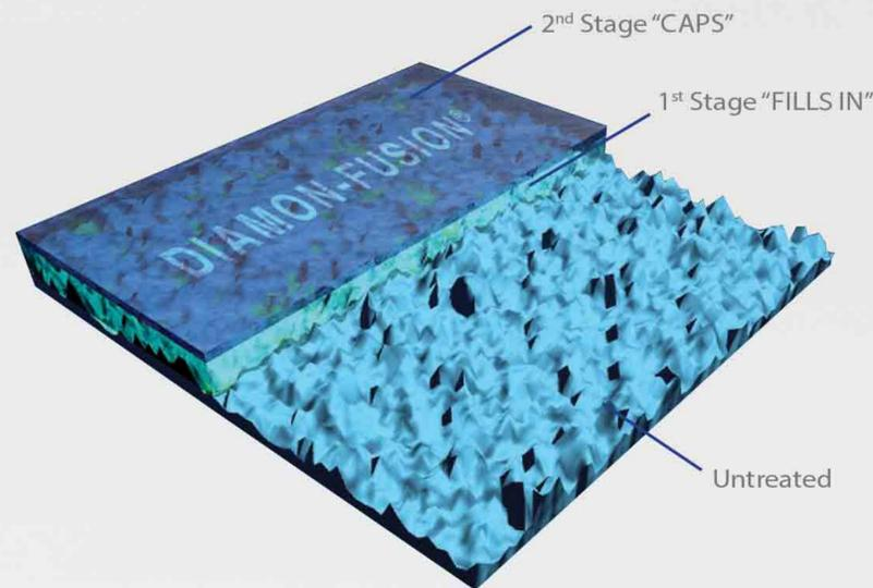
Its patented, two-step process (seen above) chemically bonds to the silica in glass filling in the peaks and valleys of the surface.
